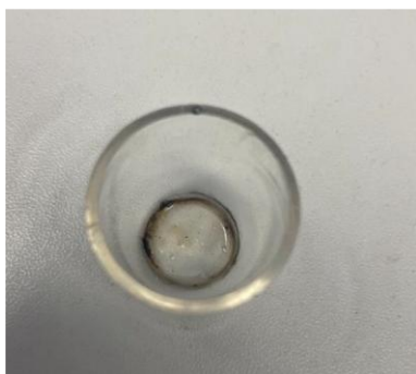
Fig. 2 View of an example crucible with sediment after combustion of a fuel sample [own photo]
