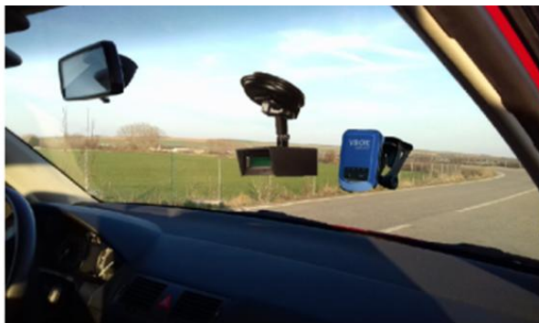
Fig. 2 XL Meter and GPS VBox measuring instruments on the vehicle windshield
