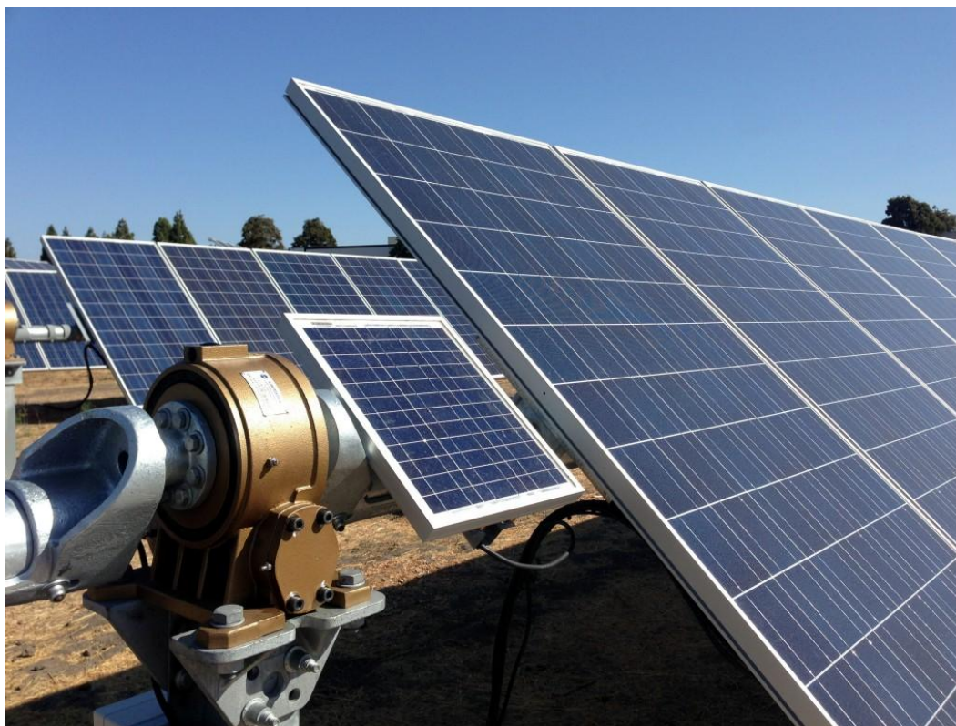
Fig. 7 Detail of the movable stand of PV panels with solar tracker and with horizontal rotating axis
