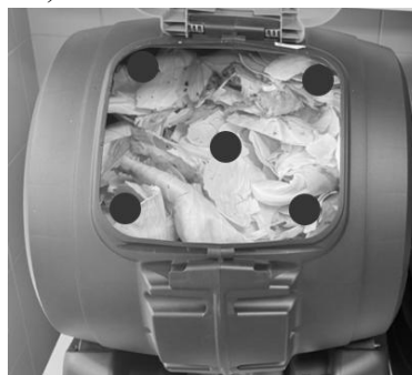
Fig. 2 Measurement points for temperature, pH, and gas concentrations
