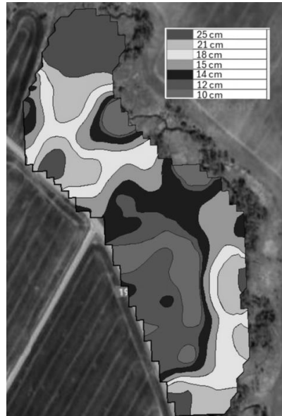
Fig. 2 Variable depth tillage map ( M 1:10,000 )
